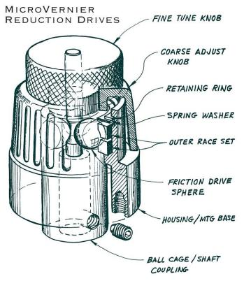
**Indexing:** Provides input shaft reduction ratios for fine tuning through a backlash planetary friction drive mechanism, offering a variety of standard ratios and mechanical interface options.
