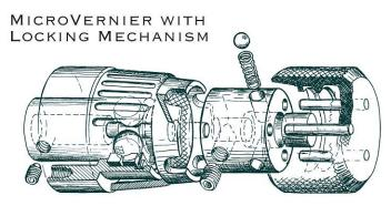
**Locking** MicroVernier is available with a friction lock mechanism to prevent inadvertent movement of the setting, integral to the unit.
